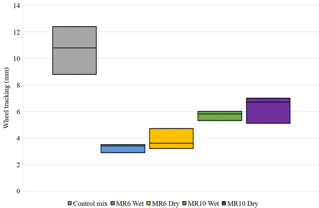
**Figure 7 Asphalt mixture deformation resistance comparison**
