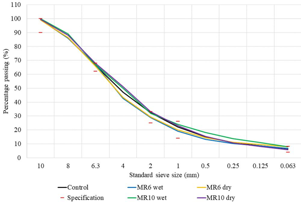
**Figure 1 Specification limits and bulk sample gradings**
