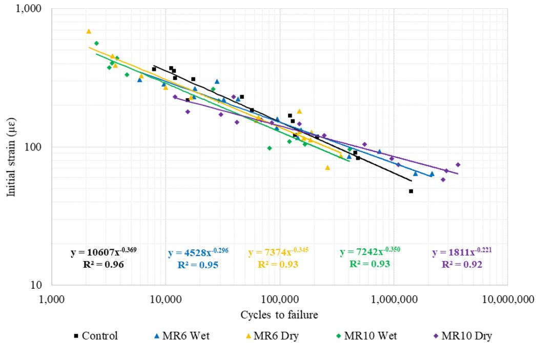
**Figure 2 Mixture fatigue results and associated relationships**
