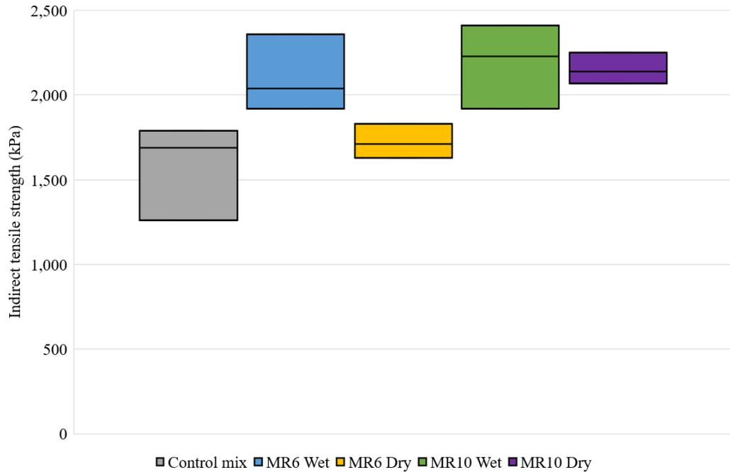
**Figure 8 Asphalt mixture tensile strength comparison**
