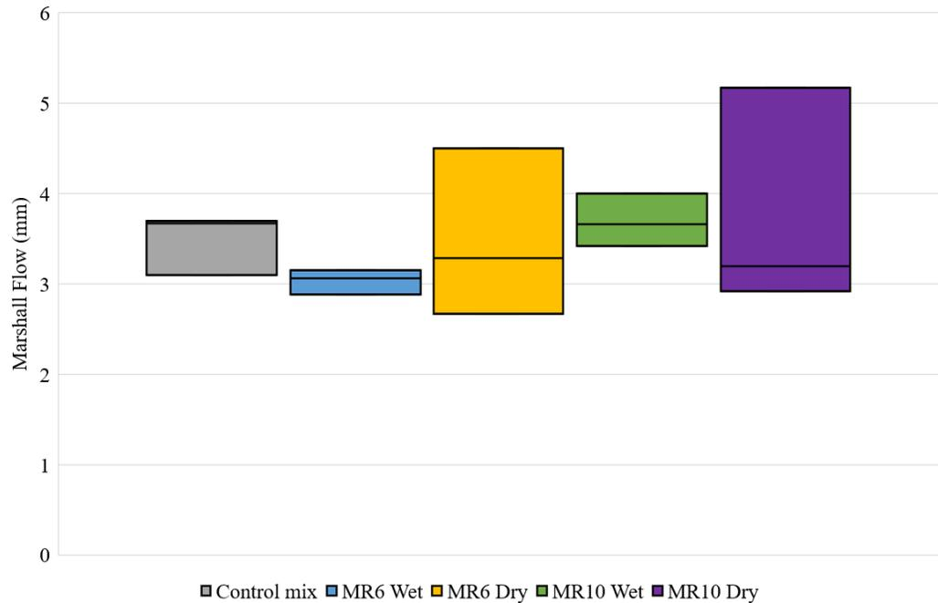
**Figure 5 Asphalt mixture Marshall Flow comparison**
