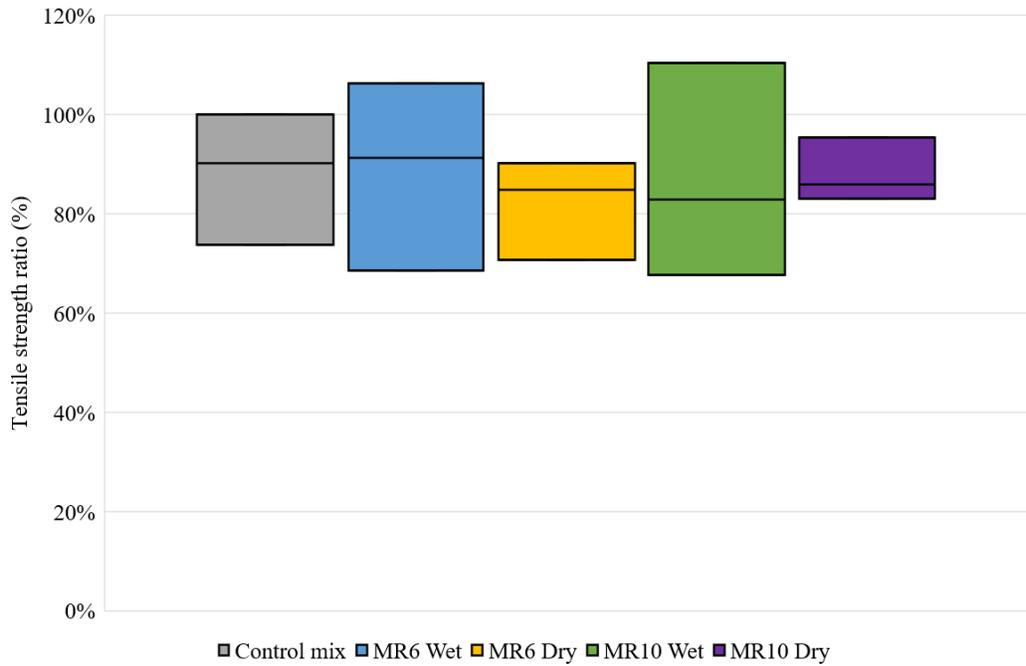
**Figure 6 Asphalt mixture moisture resistance comparison**
