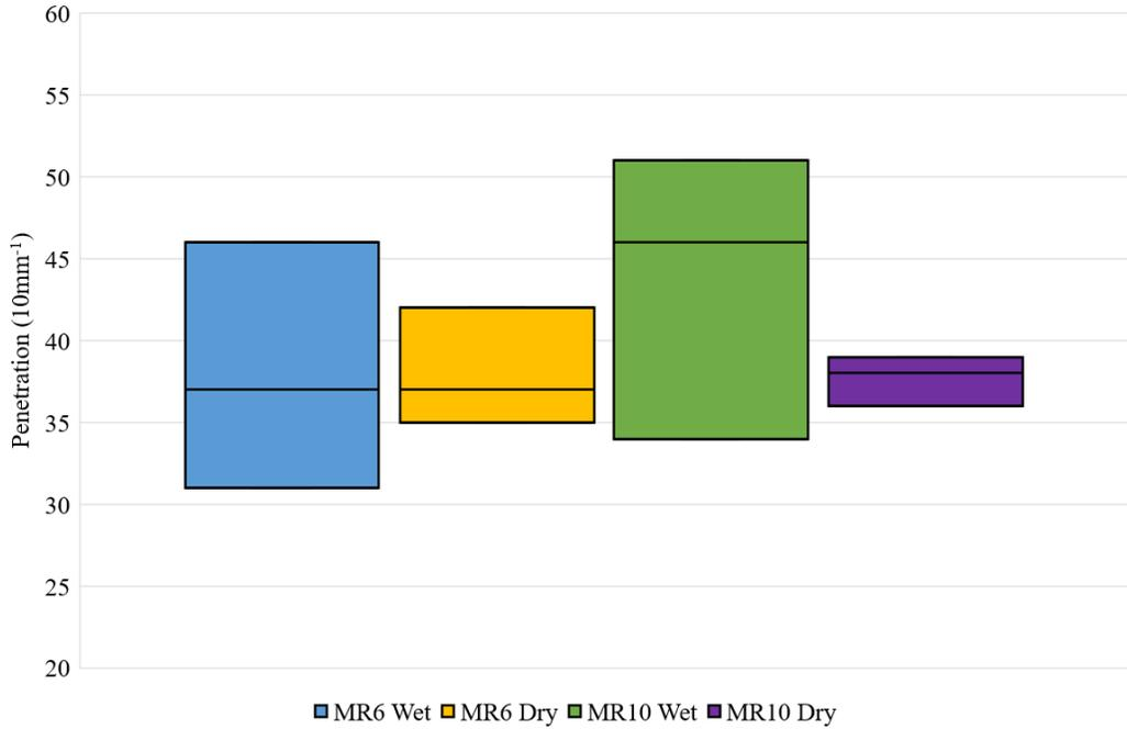
**Figure 9** Mixing effect on extracted binder penetration
