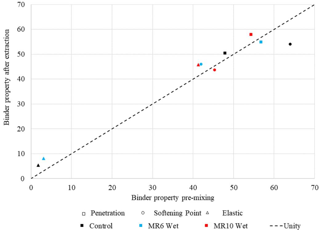
**Figure 3 Comparison of pre-mixed and extracted binder properties**
