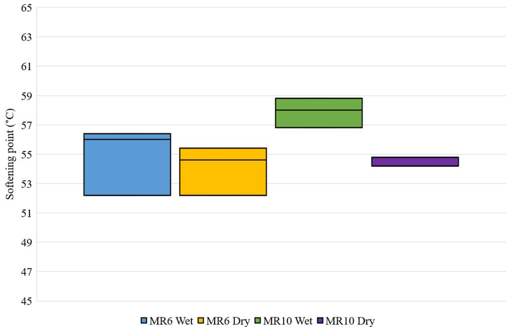
**Figure 10** Mixing effect on extracted binder softening point
