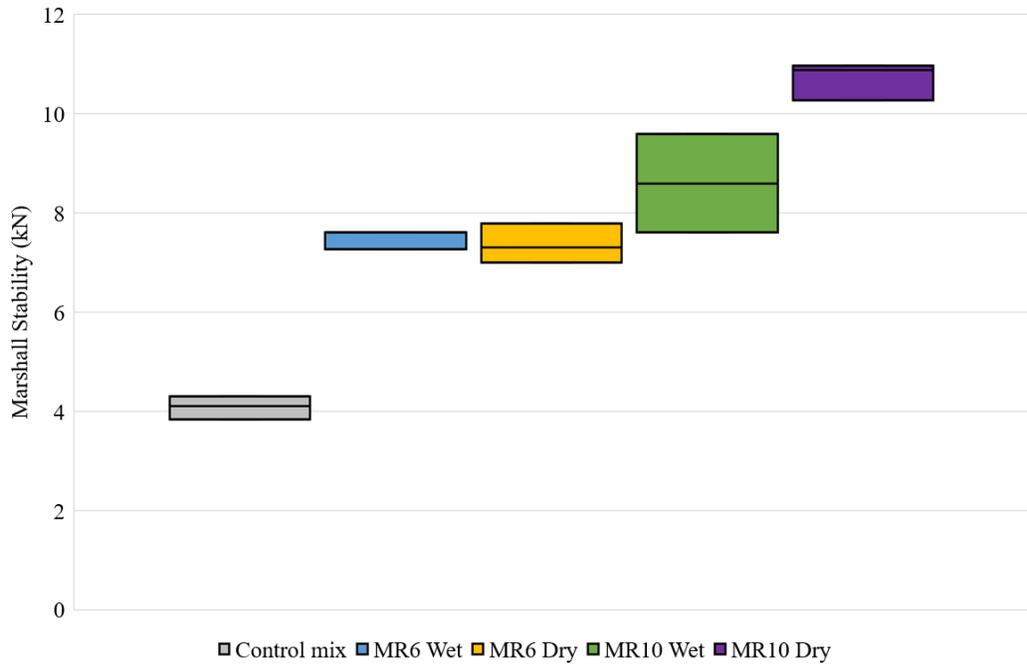
**Figure 4 Asphalt mixture Marshall Stability comparison**
