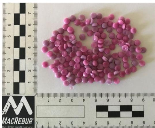
When MacRebur MR10 was then developed, it was produced in an identical pelletised form for the same reasons. In contrast, MR 8 was developed as a flaked product, as shown below, to provide the most economical bitumen extender possible.
