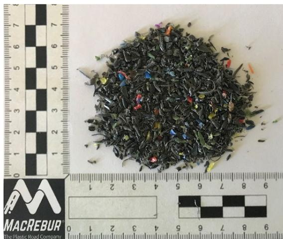
The shredded form of MR6 and MR 8 are not melted, extruded and cut into pellets, meaning they have:
