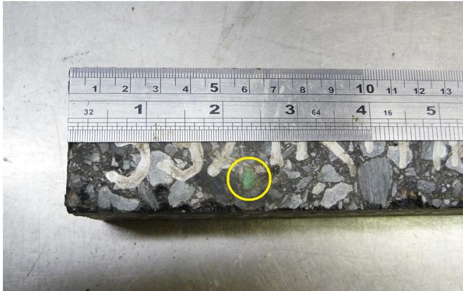
**Fig. 4 Semi-digested MR 10 pellet in fatigue beam (highlighted by yellow circle).**
