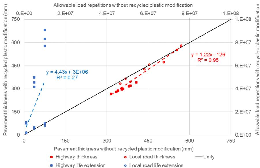
**Figure 9. Overall effect of recycled plastic modification on pavement thickness and life**
