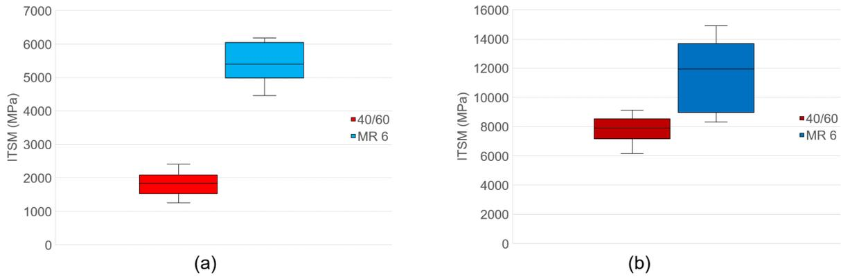
Figure 2. Laboratory (a) SMA 10 and (b) DGM 20 modulus results
