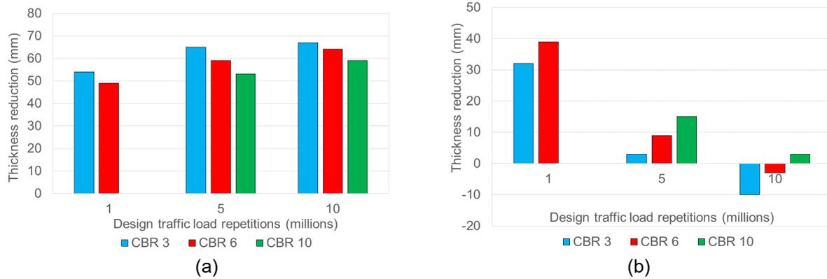
**Figure 7. Pavement thickness reduction for (a) highway and (b) local road**
