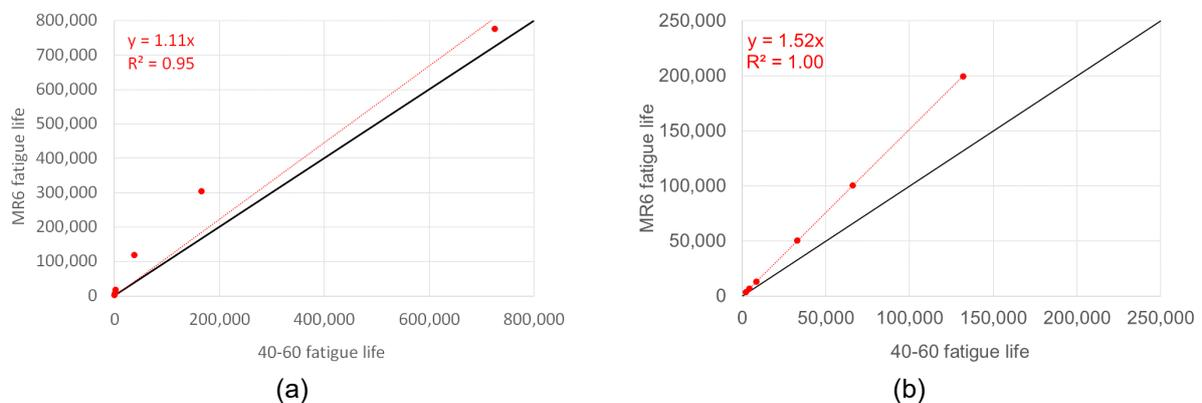
Figure 4. Laboratory (a) SMA 10 and (b) DGM 20 relative fatigue life
