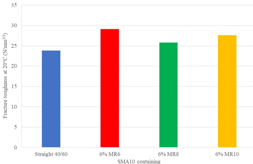
**Figure 6. Effect of recycled plastic on asphalt fracture toughness.**
