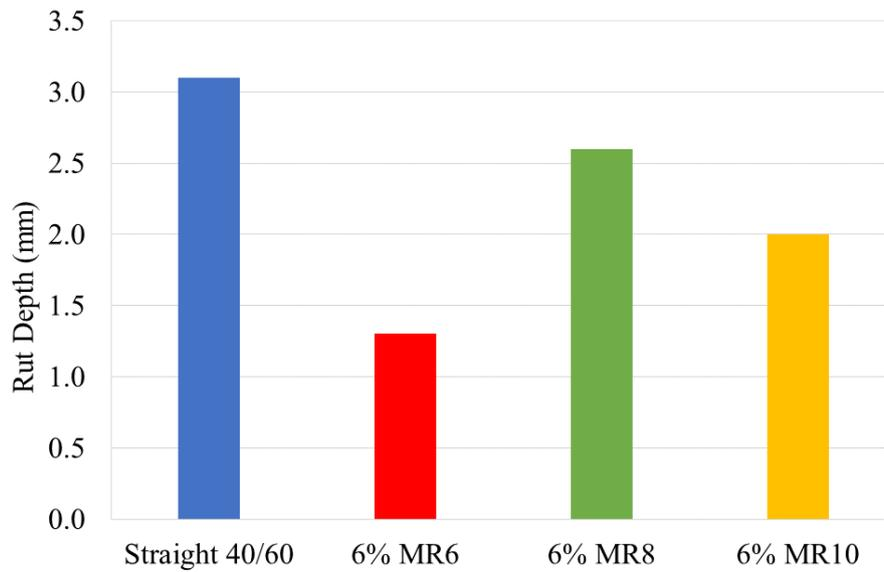
**Figure 5. Effect of recycled plastic on asphalt wheel tracking rut depth.**
