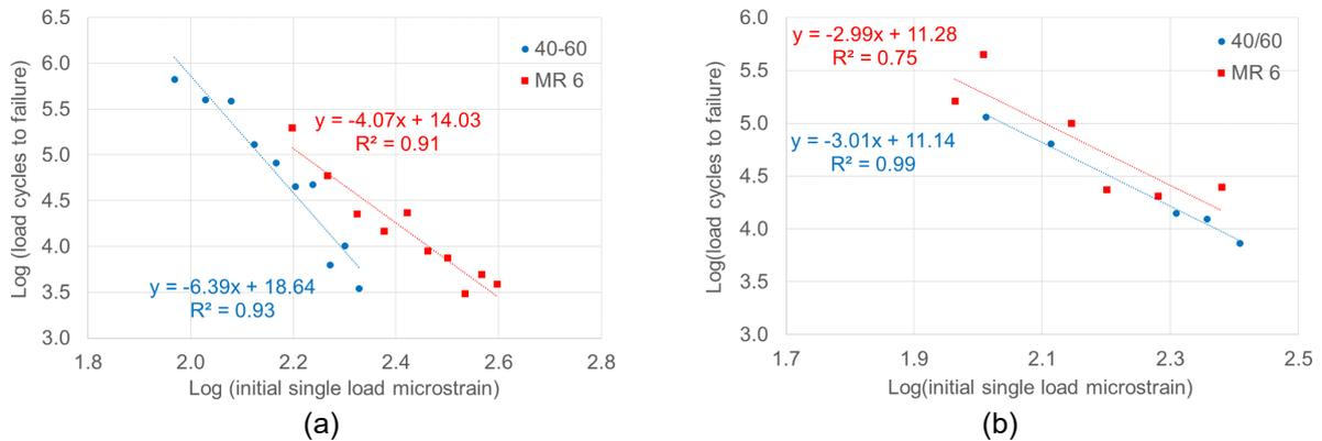
Figure 3. Laboratory (a) SMA 10 and (b) DGM 20 fatigue life results
