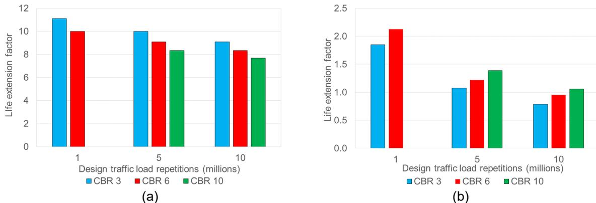
**Figure 8. Pavement life extension for (a) highway and (b) local road**
